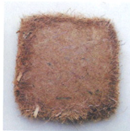
12 | Coconut Husk Boards, developed by a team at CASE, are made from post-agricultural waste and can be fabricated at multiple scales and configurations.
