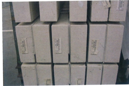
9 | Precast concrete cladding components were fabricated in Belgium and assembled in Poland to make unitized cladding panels for Allies and Morrison's Institute of Criminology (see pp. 116-23).
